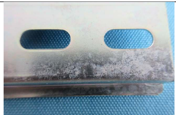
After test close-up-48h
